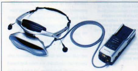
Sony's PLM-5700 (left) and the InterSense headtracker (above) together provide a hi-res virtual reality image that smoothly tracks head movement
